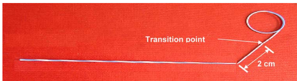
Fig. 3 The distance between fracture point and transitional point on the ZebraStent®
